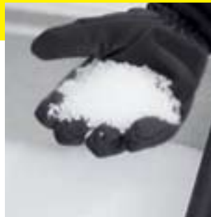
Machine is filled with 3 mm dry ice pellets.
