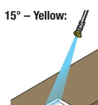
**Chiseling nozzle.** Working at a 45° angle, this nozzle works like a scraper, stripping paint, grease and grime from hard surfaces.
