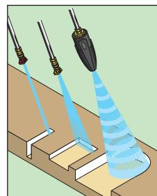
**Legacy's Revolution** gives you the best of both worlds: the deep cleaning impact of a 0° nozzle and the fast cleaning of a wide-coverage fan spray nozzle.
