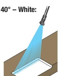
**Wash nozzle.** Its wide spray allows you to wash and rinse a large area fast. It is usually safe with most surfaces, including aluminum siding, windows and vehicles.
