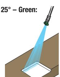
**Flushing nozzle.** The most commonly used nozzle for cleaning dirt from siding, sidewalks and metal furniture as well as for wet sweeping leaves.
