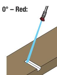
**Cutting nozzle.** It delivers a concentrated stream that can gouge or cut. It can cut stubborn stains from concrete and other hard surfaces.
