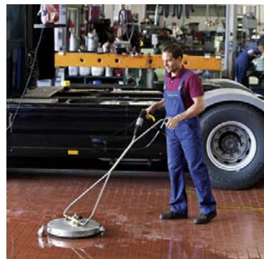
Surface cleaners offer a massive area performance and clean without splashing. They come with a plastic and stainless steel hood for hot water cleaning applications.
