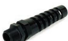
**CLAMPING SPLINES.** Various sizes and odd-shaped cables, wires and tubing can be accommodated due to overlapping diagonally split clamping splines.
