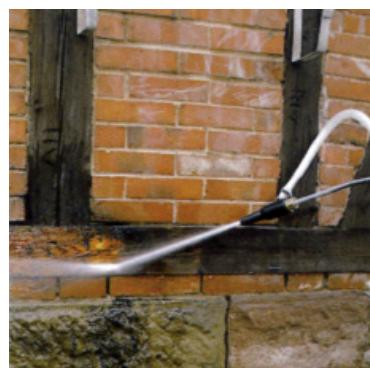
The wet blasting attachment fits easily on Kärcher high-pressure cleaner spray wands. The abrasive is sucked up into the water jet and applied with a powerful abrasive action. Ideal for removing rust, scale and paint from components as well as graffiti.
