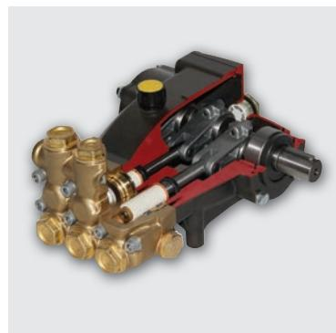
The U-Seals provide better run-dry protection, extend pump life, and allow for inlet water of up to 185°F. Kärcher K3 pumps provide a stronger crankcase with thicker mounting feet and extra-large European made tapered roller earings for longer pump life. The crankcase is reinforced and comes with the new O-ring seal for leak-free operation. Specially die cast connecting rods provide for quieter operation and longer pump life.
